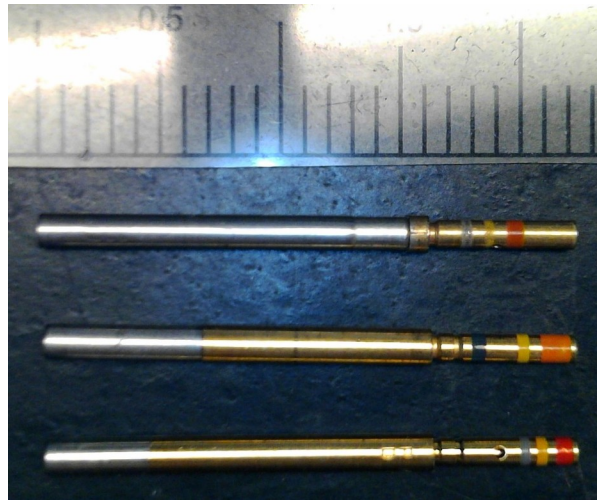
[picture: various manufacturer's versions of the M39029/56-348] Note the wide variation in the length of the steel socket
