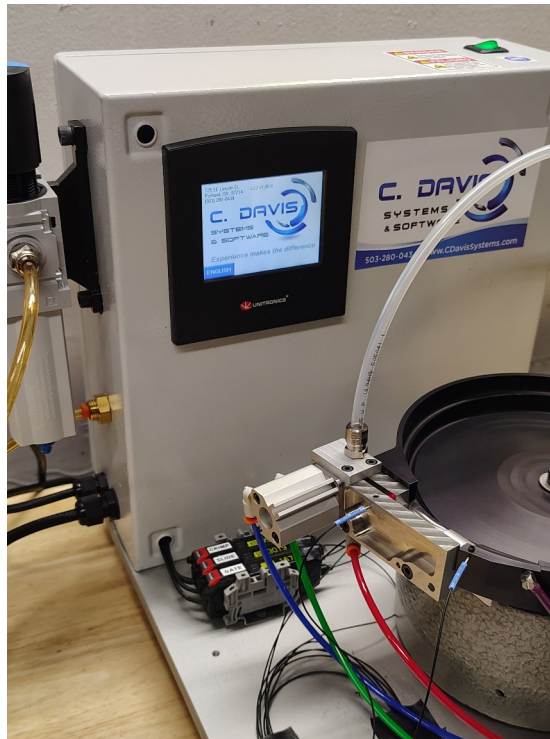
[picture: LC MACHINE with Touchscreen HMI Control Cabinet Exterior]
