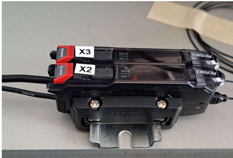
[picture: Keyence Fiber Optic Sensor Amplifiers on LC Baseplate]
