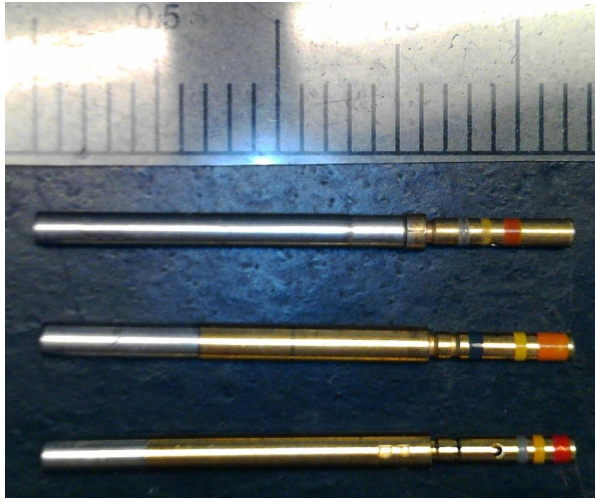
[picture: various manufacturer's versions of the M39029/56-348. Note the wide variation in the length of the steel socket]
