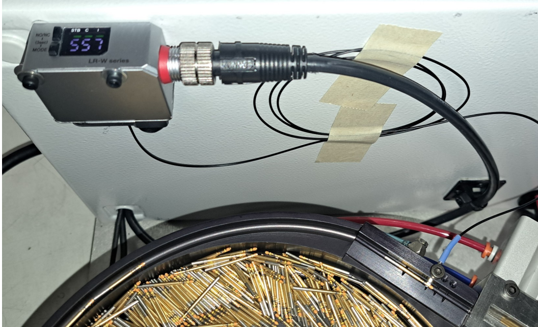
[picture: KEYENCE Color Detect module mounted on the Control Cabinet of the LC-AFM8-56-348
