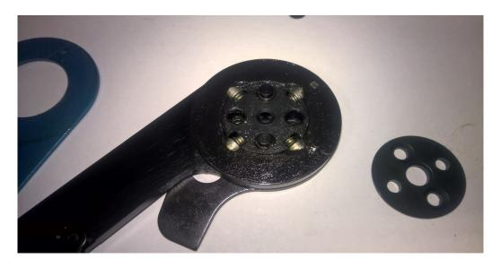
At this point you can remove the thin shims from either side of the indenter body and fully expose the indenters, cams, springs etc. This is the heart of the crimp tool.
