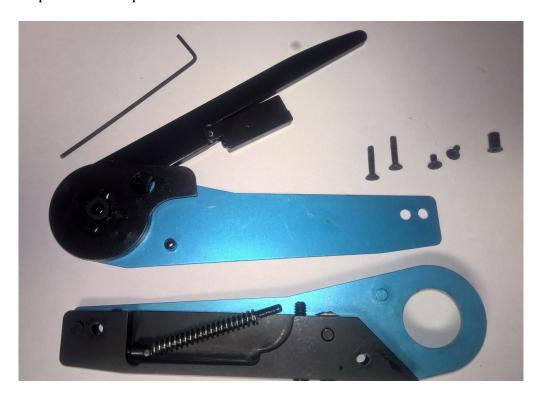
When the indenter body / handle is removed from the front side of the tool, the indenters, indenter springs and the cams of the indenter body will be exposed:
