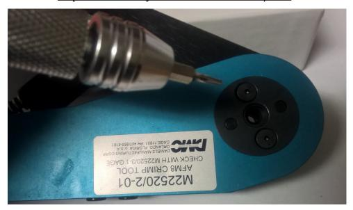
To disassemble the Daniels M22520/2-01, start with the front face of the tool (pictured above) remove the two flathead hex screws which attach the faceplate of the crimp tool to the positioner body. The faceplate may still be attached the the indenter body by two pins --if so carefully pry off the faceplace off of the indenter body.
