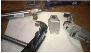
You should now be able to remove the Astro Tool's Lever Arm which contains the Indenters:
