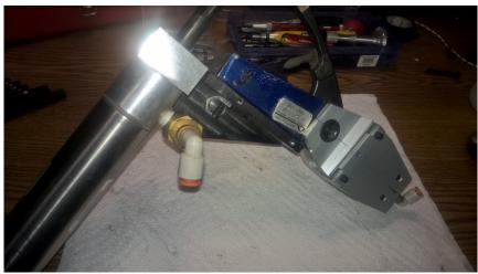
To disassemble the Astro M22520/2-01, you will first need to disassemble the crimp head itself. Start by removing the funnel jaws: first remove the Funnel Jaw Strap (or shoulder-bolts on some
