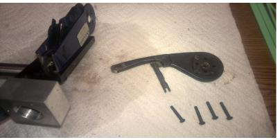
After removing the Lever Arm, remove the Indenter housing, Indenters and Springs. Be careful when removing the housing as the Indenter springs are compressed and can launch the Indenters a surprising distance. BE CAREFUL TO NOTE THE ORIENTATION OF THE INDENTOR CAM LOBES AND THE ORIENTATION OF THE LEVER ARM IN RELATION TO THEM PRIOR TO DISSASSMBLY.
