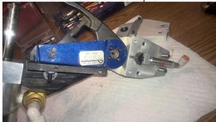
At this point the four Philips screws which hold the crimp tool to the Positioner are exposed. Unbolt the clevis from the handle of the Astro Tool and then unscrew the cylinder and the clevis. Remove the Philips screws CAREFULLY and CAREFULLY remove the Positioner from the back of the Astro Crimp tool being careful not to damage the delicate tip of the Positioner. The Astro Tool should now be attached to the baseplate, but be otherwise accessible:
