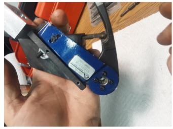
After reassembly, cycle the crimp tool manually to confirm function. The tool should articulate freely, the ratchets should engage and disengage smoothly, and the the crimp depth selector should function as before.
